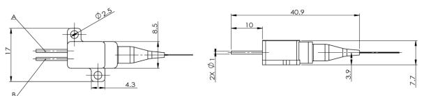
PIN OUT: PIN Description A Laser Cathode+ B Laser Anode-
